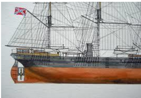
STERN SHOWING RETRACTABLE PROP
