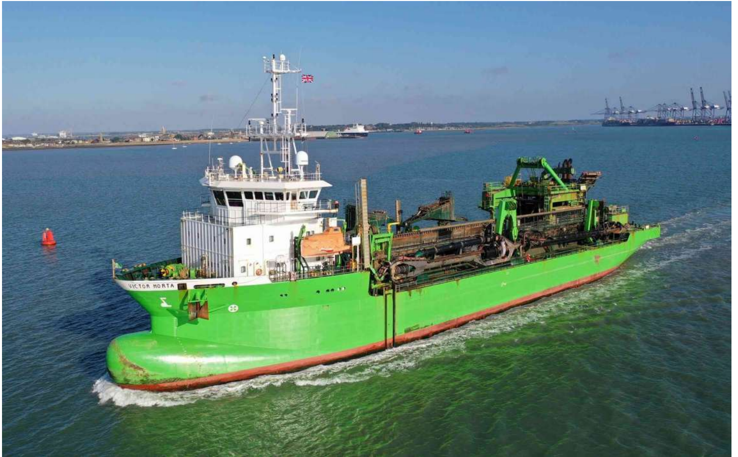
Passing through the harbour outbound from Ipswich is the aggregate dredger “ Victor Horta ”. She had self discharged her load of sea dredged aggregate earlier on the 5 th August at West Bank, Ipswich. Built for Belgium’s DEME Group in 2011 by IHC Holland dredger, Kinderdijk. (Photos contributed)
