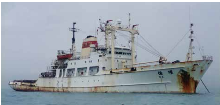
The Chinese tug DE YUE - 1979 - 200 tbp - 98,00 / 90,00 x 15,80 mld x 8,00 m - draft aft 6,94 m - two c/p props in nozzles - was one of the most powerful in the world. She carried out a number of tows under contract of Fairmount photo: coll. Job van Eijk
