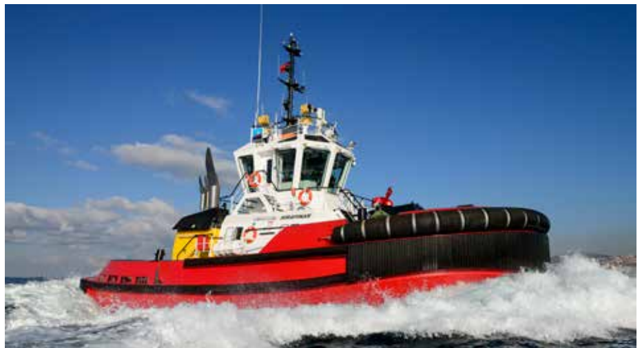
Dubai Drydocks in 2016 acquired the lead tug of a new Robert Allan / Sanmar Shipyard RAmparts-2200-SX design: DEIRA 7. Launch name SIRAPINAR is the Sanmar class name for this design. Seen here running trials. Dimensions are 22,40 m oa x 10,85 m with a draft of 4,67 m max. Depth is 4,40 m. Main engines are two Caterpillar 3512-C main engines with an output of 1.380 kW at 1.600 rpm each. Total output is 2.760 kW / 3.753 bhp. The drive train delivers a bollard pull of 46,9 tonnes ahead and 44,8 tonnes astern
