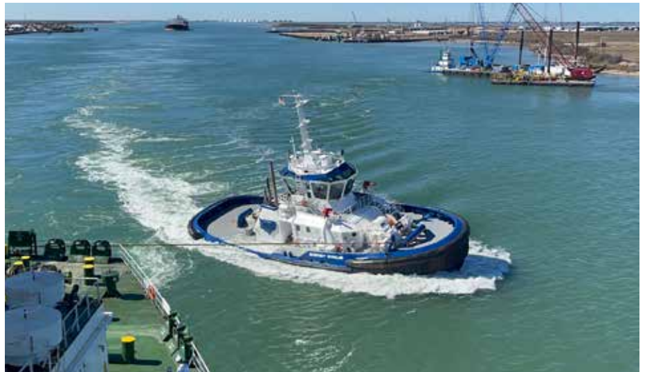
SIGNET SIRIUS in indirect steering mode
