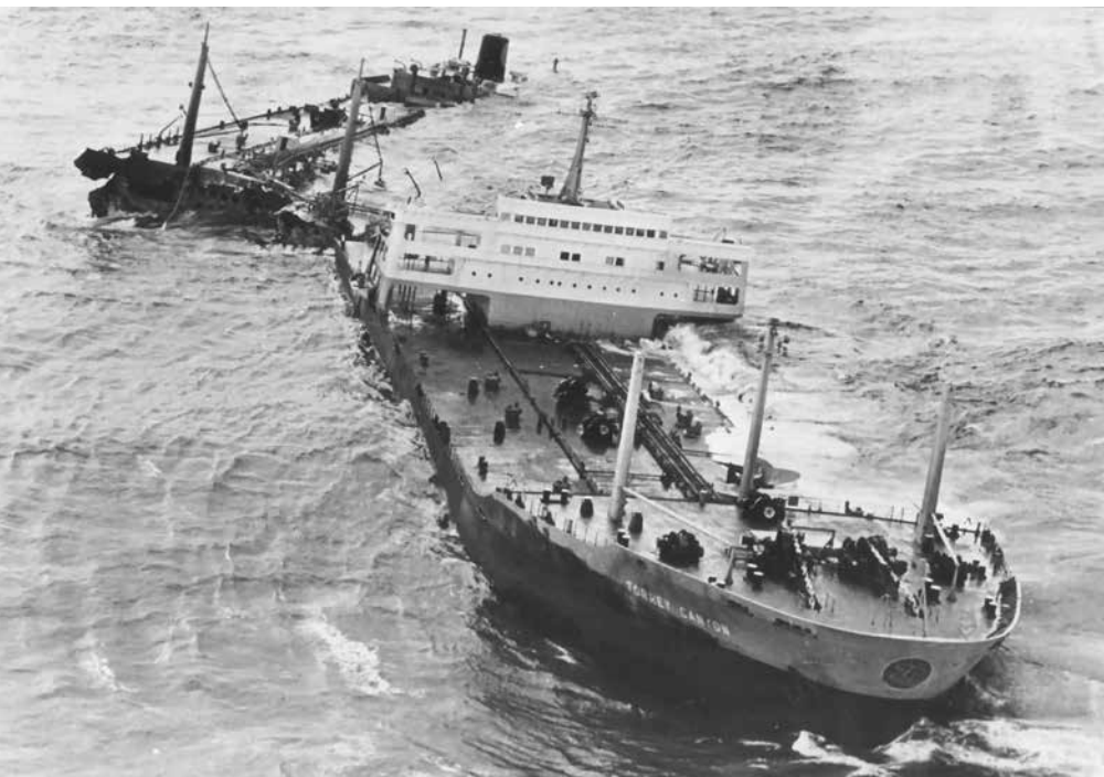
TORREY CANYON with broken back on the Seven Stones reef. A warning for the various Governments that was lost on them photo: coll. National Towing Museum, Maassluis
