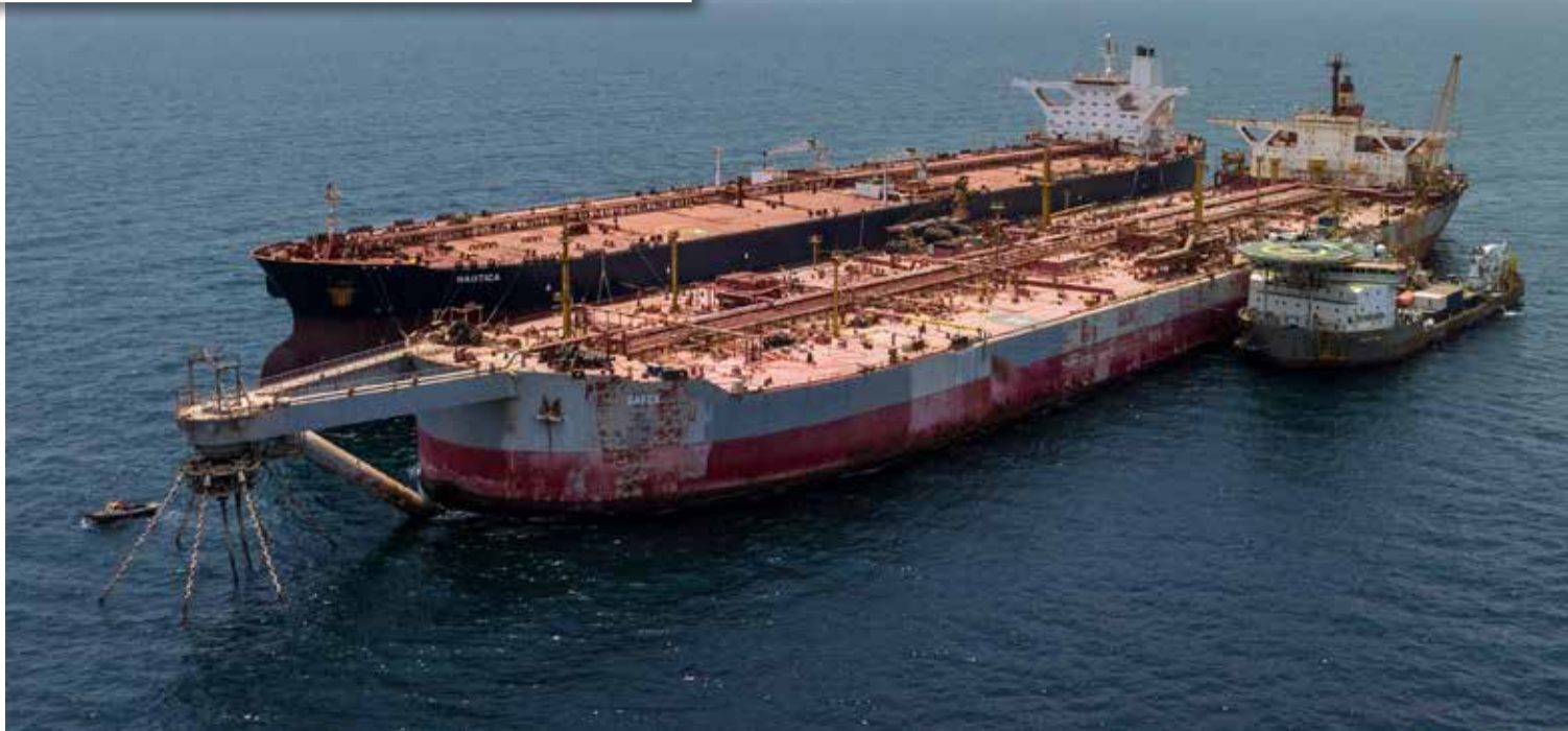
Cargo recovery operation of the SAFER FSO. SAFER was installed on location in 1988, 4,8 nm off the Hodeidah, Yemen, coast. Capacity 1,14 million barrels of light crude oil. In 2015 production was suspended due to the neighbouring war. In 2017 the inert gas systems ceased to function greatly increasing the chance of an explosion. The FSO is deemed to be beyond repair. In the picture Boskalis' NDEAVOUR alongside. She was specially outfitted for the job. Also alongside the UN-procured VLCC that will perform the ship-to-ship transfer and take the oil from SAFER
