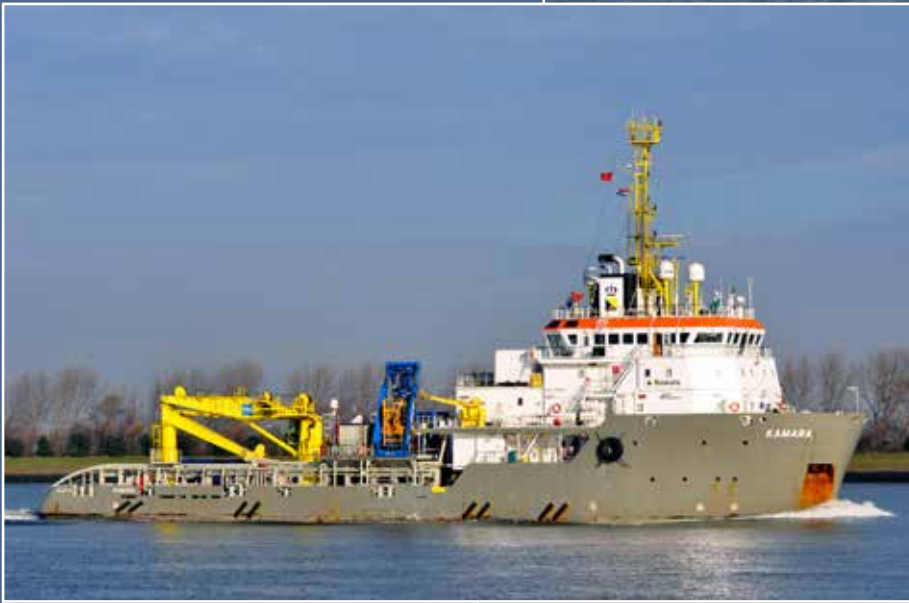
KAMARA - ex SMIT KAMARA - is an anchor-handling tug doubling as ROV support vessel photo: Ruud Zegwaard
