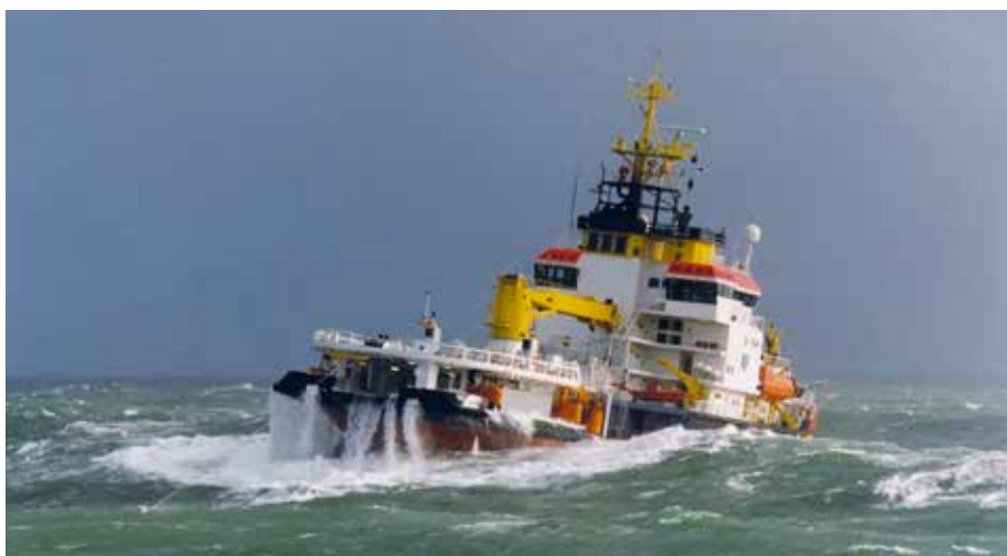
A problem of NEUWERK is the shallow draught. In a choppy North Sea with a wave height of only 3,5 metres her rudder propellers come partly clear of the water photo: Jan Mordhorst
