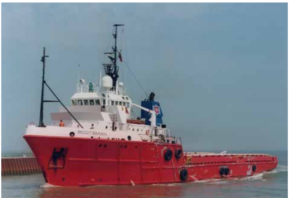
The Ulstein UT 704 design SCOTSMAN dated from 1976. The former ACTIVE PRINCE had a bollard pull of 95 tonnes
