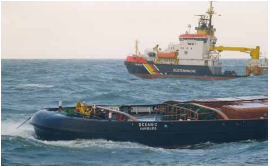
OCEANIC crew clearing the tow line. The guide pins in the tug's bulwarks are raised. In the background NEUWERK standing by photo: Jan Mordhorst
