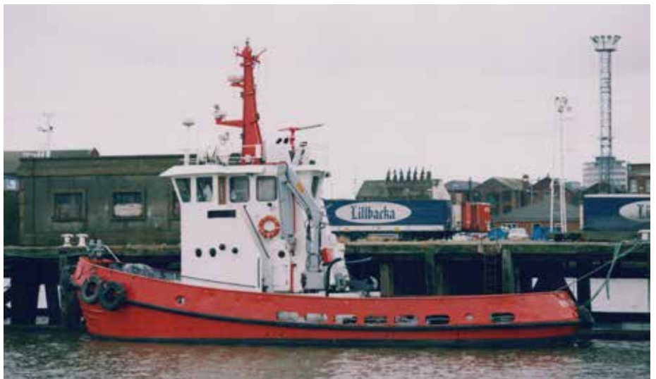
RIVERMAN is a Selmer Tug Mk-IV design built in 1977. The 12-tbp tug was acquired for smaller harbour work photo: R. & F. van der Hoek
