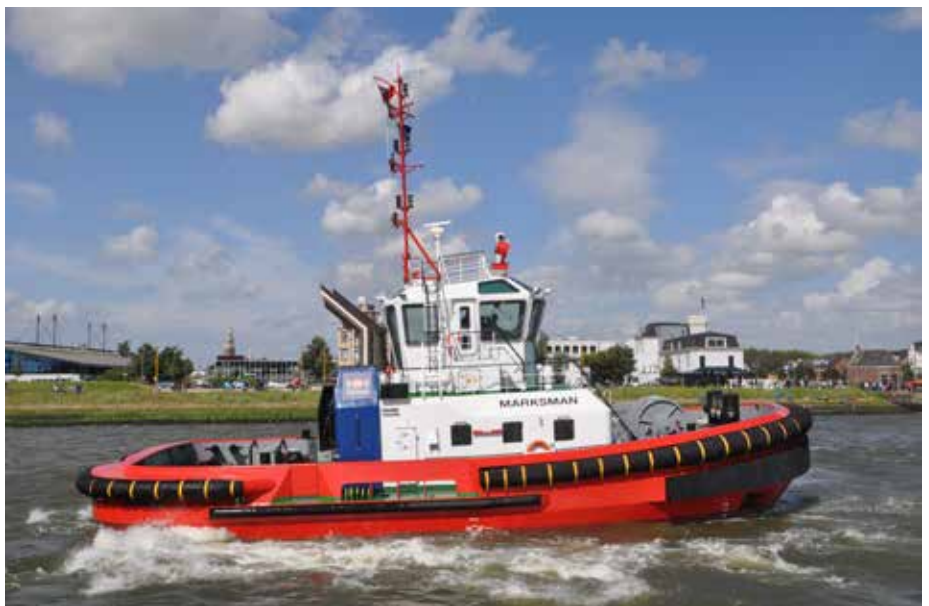
MARKSMAN was delivered in 2019 by Damen Shipyards, together with sister MANXMAN. The 72 tpb tugs are of the Damen ASD Tug 2411 design. Built by Damen Song Thu in Vietnam the tugs were finished in The Netherlands by Damen Maaskant, Stellendam
