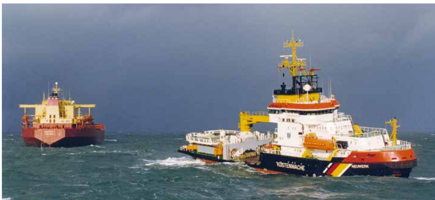
NEUWERK working up to the stern of BERGINA to hook up to the tanker's emergency towing wire
