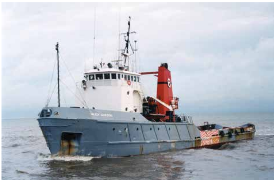
ALEX GORDON (1975 – 63 x 14,7 m – draught 4,3 m – 7.200 bhp – 75 ttp) was chartered from Specialist Marine Services for the salvage of RUBY XL and later involved in the PALLAS case
