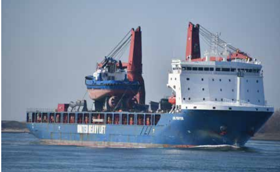
United Heavy Lift's UHL FIGHTER arrived at Rotterdam 27 March, 2025, carrying the new Damen ASD Tug 2813 FAIRPLAY-97. Built by Damen Song Cam the tug has a length of 28 m, a draught of 6 m, a bollard pull of 83 tonnes and is fitted to FiFi-1 standard. The tug is intended for operations in the Baltic photo: Ruud Zegwaard
