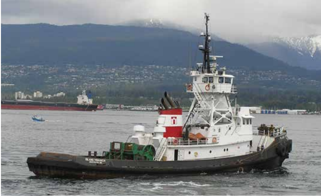
ISLAND MONARCH, 21 May, 2010, at Vancouver. The tug was built in 1966 by Star Shipyards, New Westminster, as HAROLD E JONES for Vancouver Tugboat. 1971: SEASPAN MONARCH. 1994: ISLAND MONARCH, registered under Standard Towing. The two 1994-installed EMD main engines deliver a total of 3.000 bhp (42 ttp). In 2003 fitted with 'pins' to work as an ATB pushing oil barges while her towing winch was retained photo: Nico Giltay
