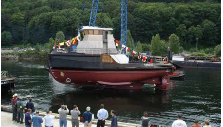
ISLAND SCOUT being 'launched'. The hull was built by Jinling Shipyard in China, then transported for finishing to Canada riding piggy-back on a newbuild barge ordered from China. Finished in Canada in 2006. 1.700 bhp, 25 tpb photo: Alan Haig-Brown
