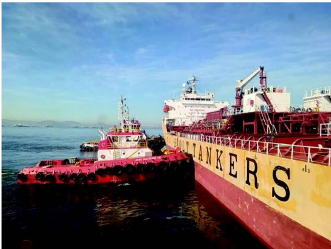
Fig 2. Tanker Stolt Kiri, 146 metres length, assisted by two powerful ASD tugs José Guilherme VIII, 32 metres length, 62 tons bollard pull and Diamante, 32 metres length, 62 tons bollard pull
