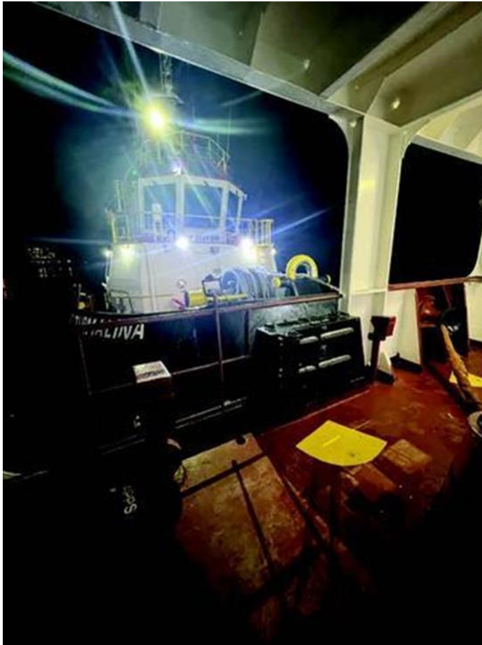
Fig 5: Ship BBC Kimberley, length 139 metres, with pushing tug Turmalina, 72 tons bollard pull. Risk of damaging ship's railing
