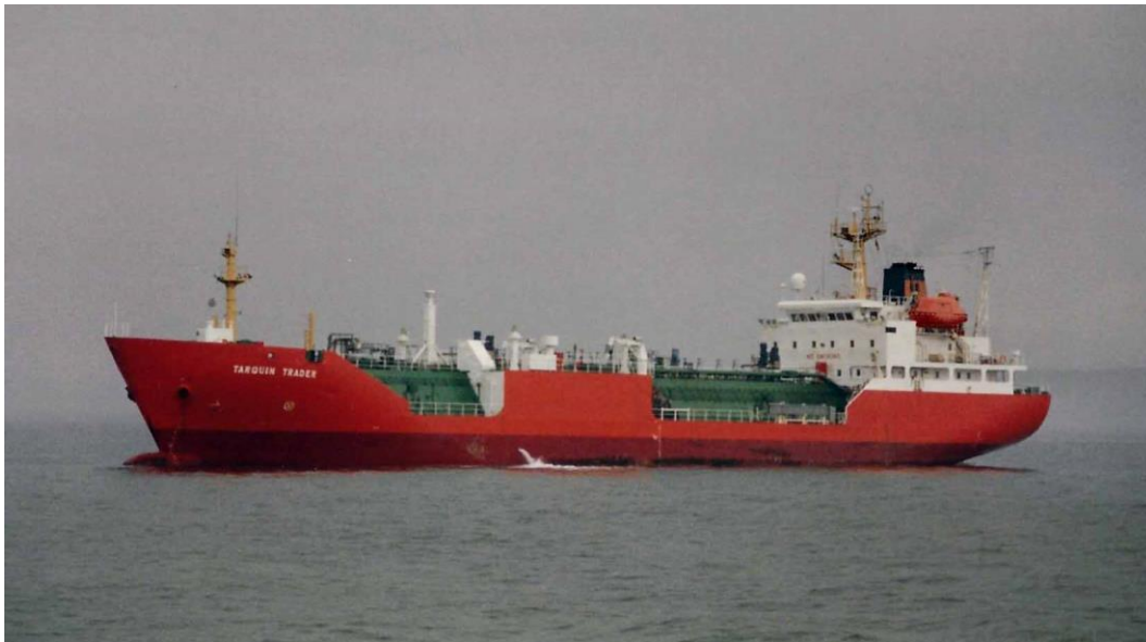
TARQUIN TRADER IMO 8716514 LPG Tanker 3,595g 4,320d Length: 98 Breadth: 15 Depth: 7.5 Draught: 6.3 (m)
