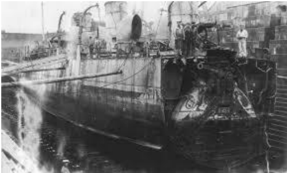
IN DRY DOCK AT CHATHAM SHOWING DAMAGE TO BOW
