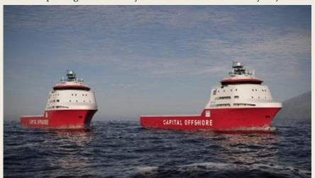
multipurpose offshore supply vessels (MPSVs) for Greek shipowner Offshore Capital Management Corp. The Z 4423 MPSV design is an 88-metre-long vessel with battery hybrid propulsion, 1000 square meter work deck, and accommodation for 60 people. The vessel is also designed with moonpool, subsea crane,
