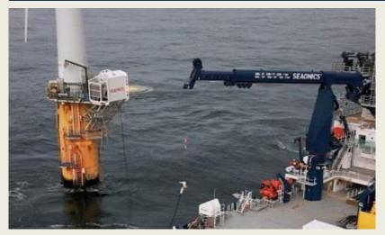
Following successful in-port and offshore prototype testing, Norwegian lifting and handling specialist Seaonics wants to commercialise its Ocean Charger solution for electric SOVs. High-voltage charging tests were conducted in port to charge the batteries on the 2023-built Rem Offshoreowned diesel-electric hybrid CSOV **REM Power** and offshore from a charging point mounted
