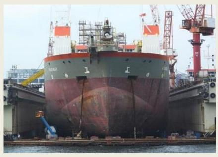
According to Boskalis, the **TSHD Fairway** undergoing major maintenance campaign, extensive involving an overhaul of all vital parts and repair or replacement where necessary. "Through periodic maintenance of our vessels we ensure that our versatile fleet can deployed as efficiently as possible," said Boskalis. The trailing suction hopper dredgers of Boskalis are oceangoing vessels that can
