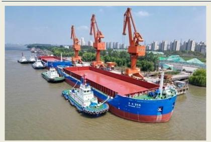
On September 8, 2024, our Jiangsu Zhenjiang Shipyard early successfully company delivered the four ships of the fourth batch of two 12000DWT badges and two 2,646 kW ASD tugboats for the "Belt and Road" project of COSCO Shipping Bulk Cargo Transportation Co., LTD. -Guinea Bauxite project. The 12000DWT badge has a length of 111 meters, a width of 30 meters, a depth of 7.5 meters, a draft of 4.88 meters, and a deadweight
