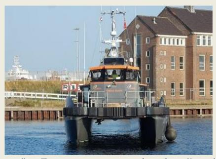
Since last Monday, the British-flagged catamaran Sword Cwind has been moored in the Wet Dock at the Willemsoord complex. It is a crew transfer vessel of the MPC22 type that is used by company Cbed transport personnel to and from offshore wind farms. The plastic-made vessel accommodate 12 passengers and 4 crew members. The Cwind Sword, built in 2014, is propelled by two Volvo Penta diesels, each driving
