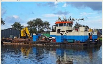
from Moerdijk to Den Helder. The Coastal Enterprise has a very shallow draft, five propellers, a strong winch and a lifting crane. Her pulling power is 16 tonnes and the maximum sailing speed is 9 knots. The work vessel, which has also been painted in the Jifmar colours in the meantime, can only be seen in Den Helder very occasionally. (Source:
