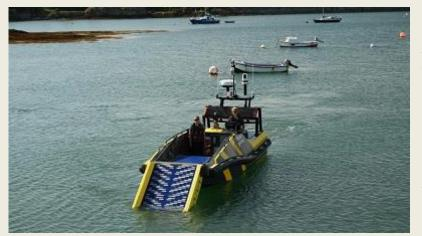
Computer processing, artificialintelligent detection software and waterjets are the technologies behind new unmanned, autonomous surface vessel dedicated finding to and recovering people in the sea. Scottish company Zelim introducing the world's first unmanned vessel for rescuing seafarers at the SMM exhibition Hamburg, Germany.
