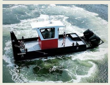
Gulf Breeze, Fla.-based Edward Maritime, a shipbuilding and repair company that provides steel fabrication services to the Eastern Seaboard and the Gulf Coast, recently launched the Raptor, a compact and versatile push boat designed specifically for small dredging and dock companies operating along the Intracoastal waterways inland rivers of the United States. According to company president Edward McDonald, the small vessel offers affordability and reliability for small
