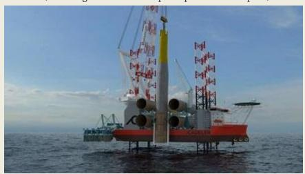
trip. It will have adjustable storage cradles that accommodate monopiles with different diameters and will be height-adjustable. The upending frame will support monopiles ranging from 80 m to 120 m in length, with what Huisman described as "enhancements for safer and more efficient upending." Key features will include a crane automation
