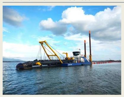
In Indonesia, the first of series CSD600 has started operation. The distinctive Cutter Suction Dredger is the first of Damen's comprehensive new dredger range to be delivered. It was transported from Rotterdam, the Netherlands to Indonesia as deck cargo on a heavy lift carrier. The stationary dredger, which has been named Jhoni 58, is working on a maintenance dredging project. The dredging operation is located at the Port of Batulicin on the island of Kalimantan. The main activities
