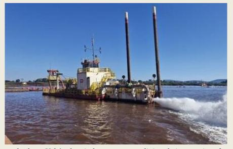
The four dredgers connect seamlessly to Vale's electrical system, streamlining their operations for
