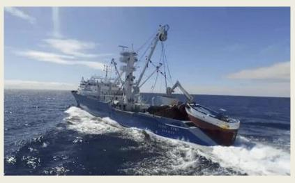
(INPESCA), based in Bermeo, and entered into service in August 2015, after its delivery by Astilleros Murueta. It is a remarkable vessel in its category, weighing 3,671 gross tons and 104 m in length. IMO code 9741085. (Source: Puente de Mando)
