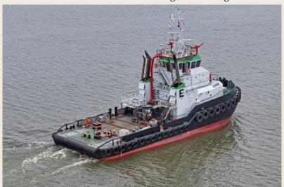
class renewal and flag change, said the Dutch marine towage and transport company. Modifications to the 70-tonne bollard pull tug (ex *DMS Osprey*) included adding a new push fender on its bow in preparation for supporting multiple types of offshore and ship-to-ship transfer operations, said the company. in chartering contracting in the towage and heavy-lift construction industry, EMAR Offshore said 2010-built
