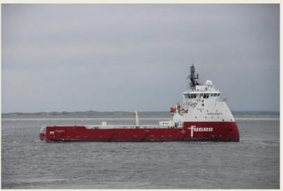
yard in Ulsteinvik, Norway. The Ulstein PX121H type ships are now equipped with a moon pool, as well as foundations for a derrick and an A-frame. Fugro will deploy the pair as geotechnical survey vessels under the flag of the Bahamas. (Source: www.maritiemdenhelder.eu)
