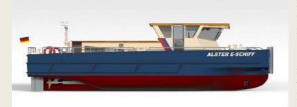
laws forbidding vessels with traditional combustion engines from operating in the waters of Hamburg beginning in 2030. Each workboat will measure 16 metres long and will have a wheelhouse that can be hydraulically lowered by 2.35 metres to allow passage
