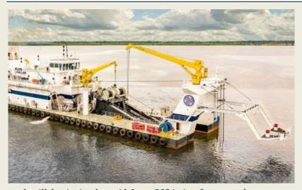
The final part of the Grand Isle Dune and Beach Construction project, dredging and beach nourishment work, is set to begin this June. According to the Town, the dredge pipeline currently being assembled along the beach will be used to pump sand along the beach and dune starting at the western end of the beach and moving eastward. Grand Isle city officials anticipate that the pumping of
