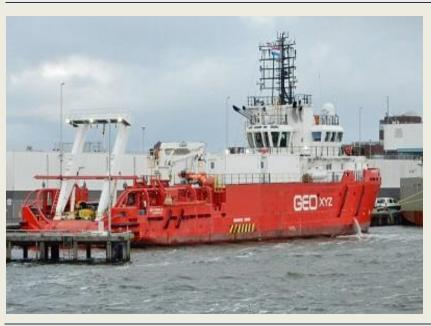
Tuesday evening, almost 54 meter long GEO Ocean VI moored behind the Blue Port Center. The striking survey vessel of GEO xyz from Zwevegem, Belgium, had come to Den Helder from Grimsby. The ship was built in 2014 under the name **Bourbon** Grebe as a so-called seismic support vessel for the French shipping company Bourbon CGG. It was later taken over by GEO xyz and converted into a multifunctional survey vessel with hybrid propulsion. The
