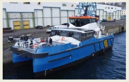
This is a smart functional little aluminium catamaran that boasts a number of interesting features, especially the aft location of its wheelhouse. Built in Piriou's busy Vietnam yard, the vessel is very adaptably multi-role. It is safe, fast, comfortable, economical and very capable. "It was the first crewboat we designed and built in-house after having delivered several other crewboats in previous years,"
