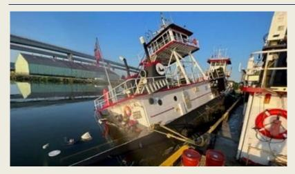
An open overboard shutoff valve and a failed check valve led to the sinking of a laid-up towboat at a yard in New Orleans last year, the NTSB has concluded. At about 0600 in the morning on June 25, 2023, an employee found the towboat Joanne Marie listing heavily and partially flooded at the Bollinger Quick Repair Shipyard outside New Orleans.
