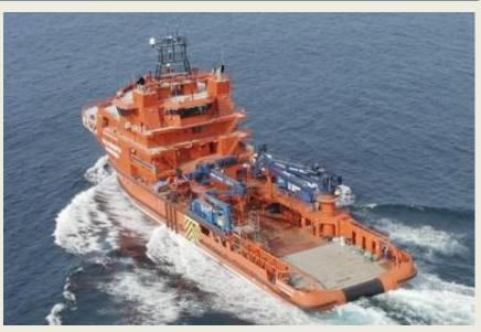
gear, equipment for cleaning up oil spills, a large open aft deck, two knuckle jib boom cranes, and flight deck and hangar facilities for use with unmanned aerial vehicles. Two 2,953kW main
