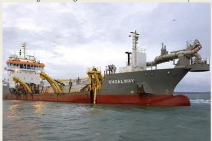
and grid operators. And for that job Boskalis' hopper dredger **Shoalway** proved to be ideally suited. Because the vessel can both extract and backfill sand via its suction pipe, the **Shoalway** was able to precisely deposit the new sand berm on the cable route, making it resistant to erosion for years to come. (Source: Dredging Today)
