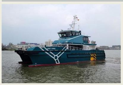
Experienced Japanese operator Tokyo Kisen Co Ltd has taken delivery of the first of two new bespoke crew transfer vessels (CTVs) to service Japan's growing offshore wind energy sector. Constructed by Cheoy Lee shipyard in China, the first vessel successfully completed sea trials in late 2024. The two Class NK 26-metre catamaran CTVs have been developed with Tokyo Kisen to comply with strict local regulations. The design of the
