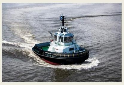
SCHOTTEL is to equip four new 1810-series ASD stock tugs from the Dutch Damen Group with the SCHOTTEL RudderPropeller type SRP 270. The new multi-purpose tugs will have a bollard pull of 30 tonnes each and ensure excellent manoeuvrability with a compact size of just 18.25 metres in length and a beam of 10.23 metres. Greatest possible performance in an extremely compact vessel. The power rating of the SRP 270 amounts to 1,000 kilowatts per
