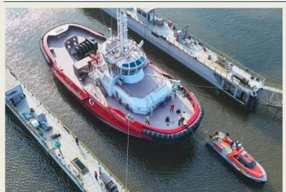
On February 27th, 2024, the world's first Voith propelled tractor tug with LNG dual fuel propulsion was successfully launched by Uzmar Shipyard in Istanbul, Turkey. Named the Sultanhani, this is the first of two hulls being built for Turkish tug operator BOTAS to Robert Allan Ltd.'s TRAktor V3900-DF design. A first of its kind design, the TRAktor V3900-DF builds on Robert Allan Ltd.'s extensive experience designing both Voith
