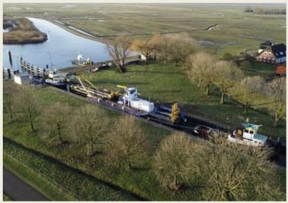
crew on location as well as dredge spares to facilitate maintenance duties. The distinctive CSD600, which is being shipped as deck cargo at present, is a brand-new type of dismountable dredger, recently added to the Damen standard range of dredgers. The dredger has a cutter power of 250kW and a maximum dredging depth of -16m. (*Dredging Today*)
