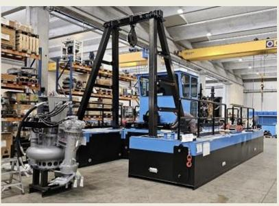
dredgers are ideal for dredging operations in difficult-to-access places, such as mining basins and artificial reservoirs. They are dredgers that are easy to transport and assemble, characteristics that make them able to reach even the most remote places. *(Source: Dredging Today)*
