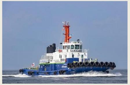
Tugboat Sakigake, also known as the world's first commercial-use ammoniafuelled vessel, wrapped up demonstration voyage, its reaching a greenhouse gas (GHG) emission reduction of up to approximately 95%, the vessel's operator NYK Line has reported. The reduction emission was recorded during the threedemonstration month voyage which commenced after the tugboat was
