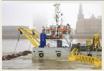
The vessel **Pieter Coecke** is active in the river Scheldt and the Port of Antwerp, sweep dredging and clearing debris and oil. It does so on behalf of the Department of Mobility and Public Works of the Flemish government. Thanks to its new engines, equipped with ULEv technology, emissions are now reduced by 85% to even 98%. At the end of 2024, the Pieter Coecke underwent maintenance at Damen Shiprepair Vlissingen, where it was fitted
