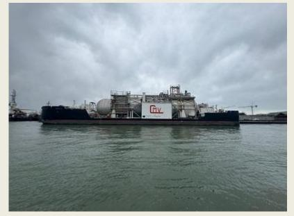
This integrated tug and barge system represented the first example of made in Italy equipment for naval bunkering; the floating barge is equipped with tanks with a capacity of 4,000 cubic meters of gas and 1,276 marine diesel oil and will be towed by a tug with dual-fuel LNG diesel power supply that can operate autonomously. As for the technical characteristics, the new construction is composed, as mentioned, of a platform called 'cargo unit', 109 metres long and 26.7 metres wide, equipped with
