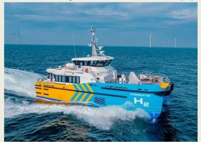
that significantly enhance crew comfort and operational efficiency. Developed through inhouse innovation, the MK5 design feedback incorporates and from experience the daily operations of our fleet and offers further optimised seakeeping capabilities, larger deck space, and provisions for increased hydrogen storage. With an overall length of 27 meters, an optimised hull shape, increased width, and elevated freeboard, these vessels ensure greater accessibility and
