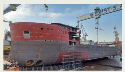
Nexans says construction of Nexans Electra, the company's third cable-laying vessel, which is due to be delivered in 2026, reached has а maior construction milestone. The hull of the vessel, which is being built at Crist shipyard in Poland, is now fully assembled, and has been moved to the dry dock at the yard for final positioning, before the dock is
