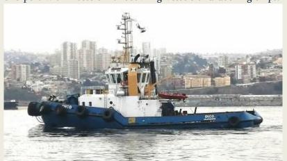
commercially viable. Ultratug is using MAHI's Remote Operation solution on 2010-built, 32-m tug **Enco** to reduce manning in the wheelhouse during long coastal voyages to service remote ports. This uses onboard computers, sensors and software for semi-autonomous navigation with monitoring and command from an onshore operations centre in Vina Del Mar, Chile. It is likely
