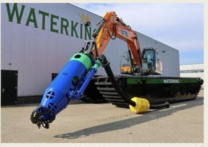
Dutch Waterking, manufacturer of dredging equipment, has proudly presented the world's first electric amphibious dredging set. In collaboration with Staad Groep, Waterking assembled a 35-tonne electric amphibious excavator – the WK 350 NG-E, while Damen provided the E-DOP 150 to complete the emission free set. According to Waterking, Fusion Energy EU a brand of Staad Group – developed a Powerbox 400
