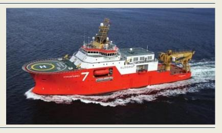
featuring VS 471 design. The versatile Inspection, Maintenance and Repair (IMR) vessel is capable of accommodation 90 people. In mid-2024, Subsea7 extended the contract for the vessels with Solstad Offshore, exercising the 2025 optional charter, with no further options. **Normand Subsea** CSV is owned by Solstad Maritime Holding, in which Solstad Offshore holds 27.3%. (*Source: MarineLink*)
