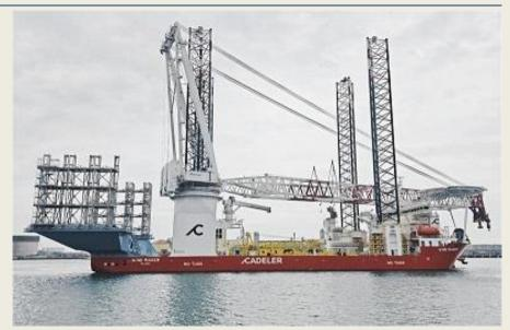
farms, said Ørsted, the developer of the project. The jack-up wind turbine installation vessel was delivered by South Korean shipbuilder Hanwha Ocean to Cadeler in January 2025. Outfitted with a 2,600-tonne main crane, Wind Maker enables the stable installation and maintenance of heavy
