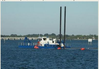
Inlet. The company will now begin dredging approximately 215,000 cubic yards of beachcompatible sand from designated sand trap and adjacent navigation channel located within Sebastian Inlet. Sand is set to be placed on the downdrift beaches between the state park's day use beach on the south side of the inlet and McLarty Treasure Museum. The project is necessary for the Sebastian Inlet District to meet its requirement to bypass sand that migrates into the inlet
