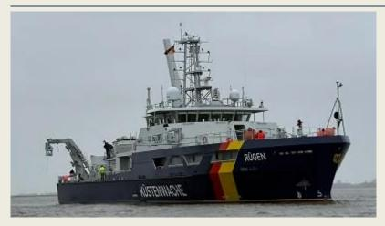
The German Federal Customs Service (Bundeszollverwaltung) recently began operating a new multi-purpose vessel. Built by local shipyard Fassmer, the vessel has been named **Rügen** after an island in the Baltic Sea. It is the largest vessel in the current active Bundeszollverwaltung fleet with a length of 67 metres (220 feet) and a beam of 12.7 metres (41.7 feet). A draught of 2.85 metres (9.35
