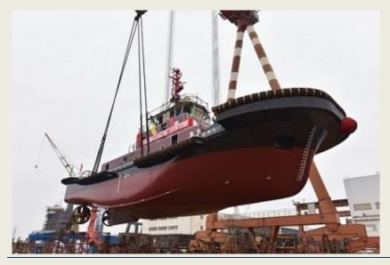
On 14th February, 2025, one unit of 2,942kW ASD tugboat built by Jiangsu Zhenjiang Shipyard for Jiaxing and named "JIA GANG TUO 17" has been launched. Representatives from owner company attended the ceremony. (Source: Jiangsu Zhenjiang Shipyard)
