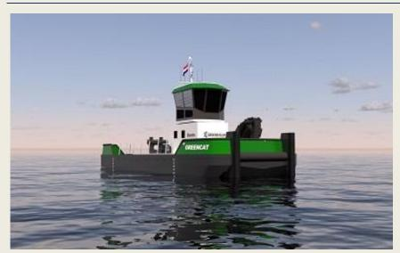
We are proud to present our newest electric work vessel: the **GreenCat**. Building on the proven success of our EasyWorker 2080, the **GreenCat** has been further developed to set a new standard in sustainable innovation. The GreenCat revolutionary features a battery exchange system capable of accommodating up to six 400 kWh batteries. These batteries provide
