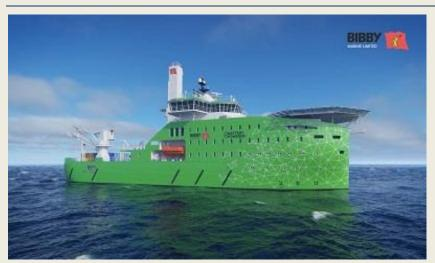
Kongsberg Maritime has secured a contract to supply an integrated package of equipment for Bibby Marine's new electric Commissioning Operation Service (eCSOV), the world's first fully-electric offshore vessel. Kongsberg Maritime will provide full-electric rimdrive propulsion with azimuth and tunnel thrusters. The scope of supply also
