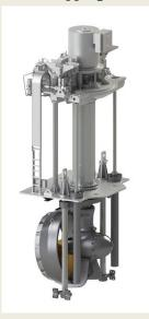
required operation profiles of the LNG bunkering vessels. *Fully 360-degree steerable propulsion unit* The propulsion packages also each include a SCHOTTEL Retractable RudderPropeller type SRP 380 R (1,300 kW with a propeller diameter of 2,200 mm). When extended, the SRP-R functions as a fully 360-degree steerable propulsion unit. It allows maximum manoeuvrability, high propulsion
