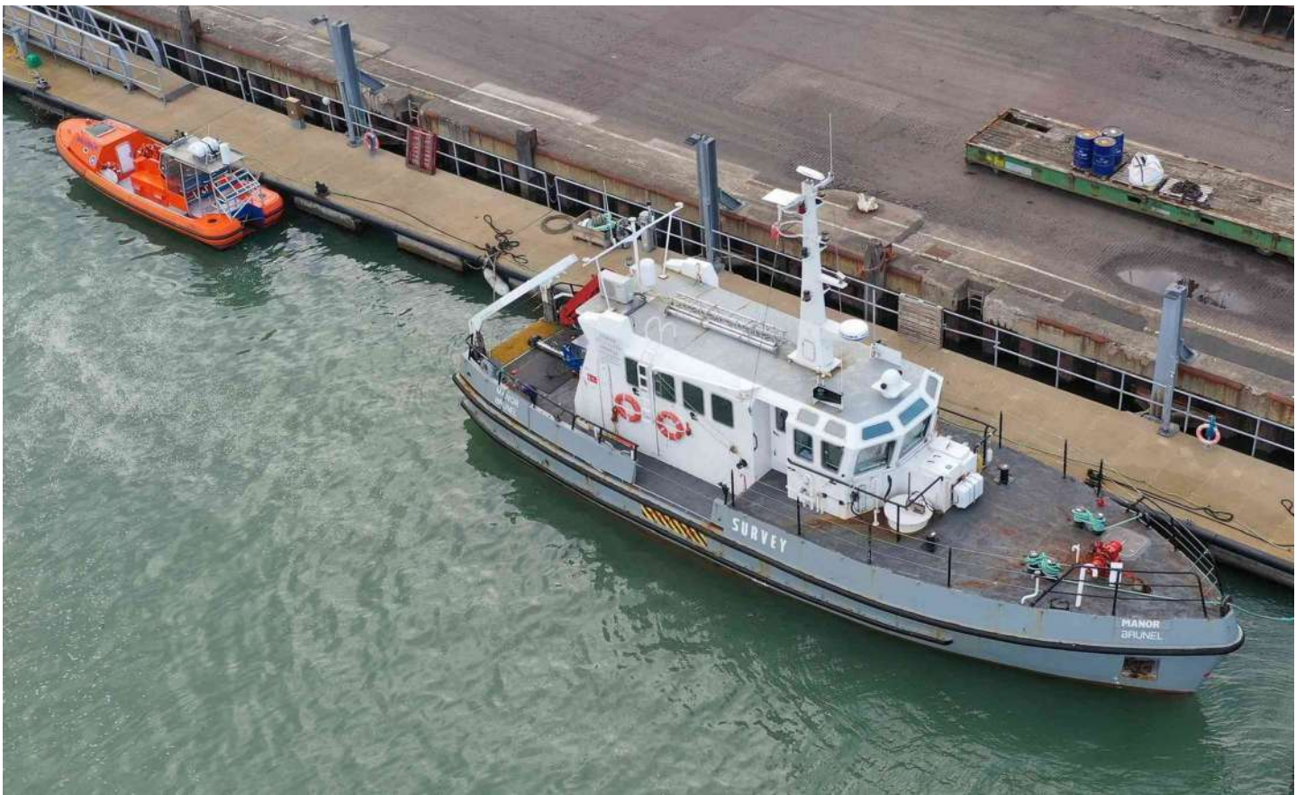
Seen at Harwich Navyard wharf is “ Manor Brunel ” a survey vessel belonging to OEG renewables of Portland. Powered by two Cummins diesels she is capable of fourteen knots. Purchased in May 2021 and upgraded, she was formerly the “ Isambard Brunel ” previously owned by the Bristol Port Company she was built in Bristol in 2008. She left for Lowestoft on 30 th August. To her stern is the “ Balvenis ”, about which information is sort. (Photo contributed)
