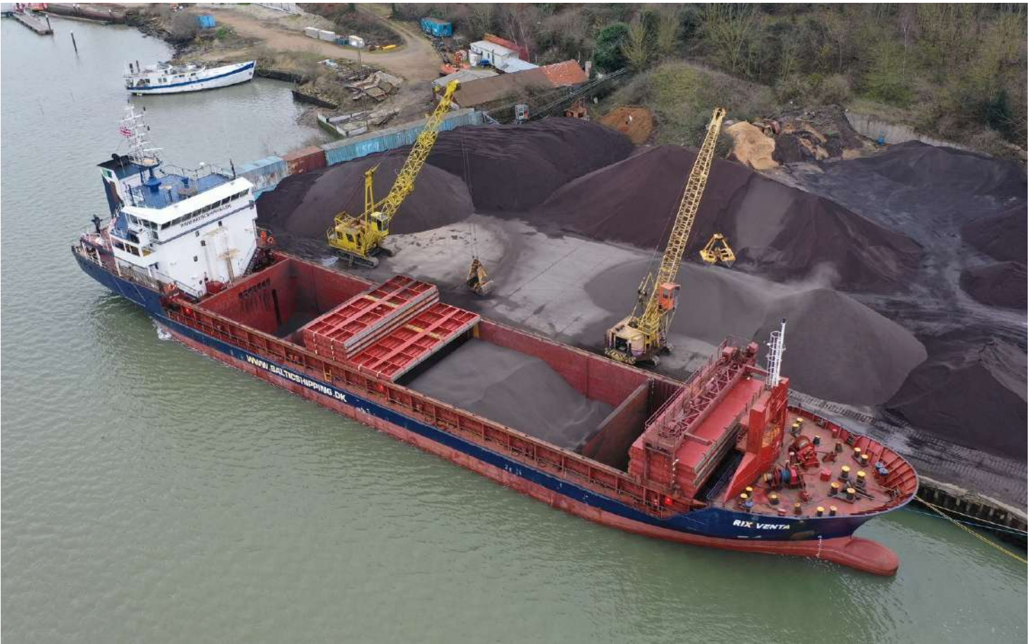
Discharge continues from the middle of the hold as witnessed by a high flying drone. (Photo contributed)
