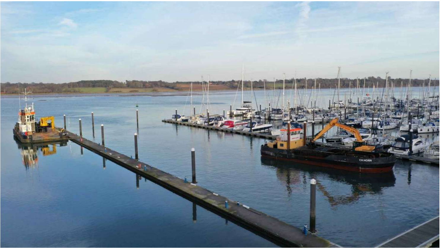
Whilst “Wind Lass” lays by on the pontoon at Woolverstone “C.H. Horn” is hard at work. She was built by James Cook at Wivenhoe in 1968 and has a Priestmann 500 grab. (Photo contributed)
