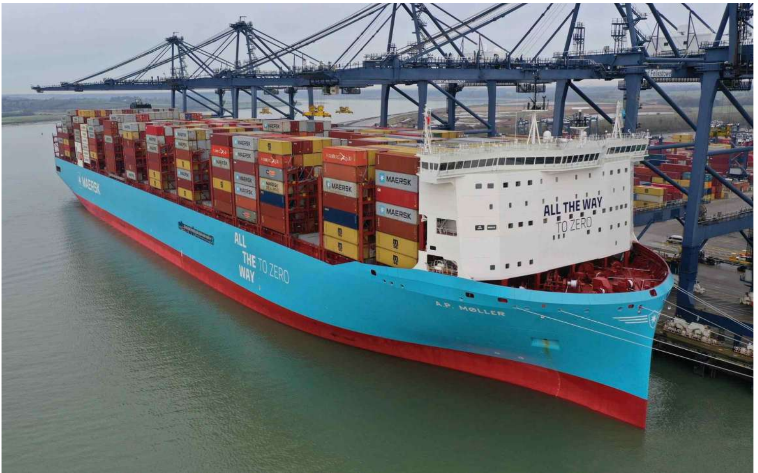
“A. P. Moller” at Trinity seven, Felixstowe on 4 th January, during her maiden voyage. She had arrived the previous day from Singapore, calling at Tanjung Pelepas, Colombo and Tanger Med on the way. Capable of 15,146 TEU the 350 metre long ship has a design speed of 21 knots and was completed in November 2024 by Hyundai Heavy Industries. (Photo contributed)
