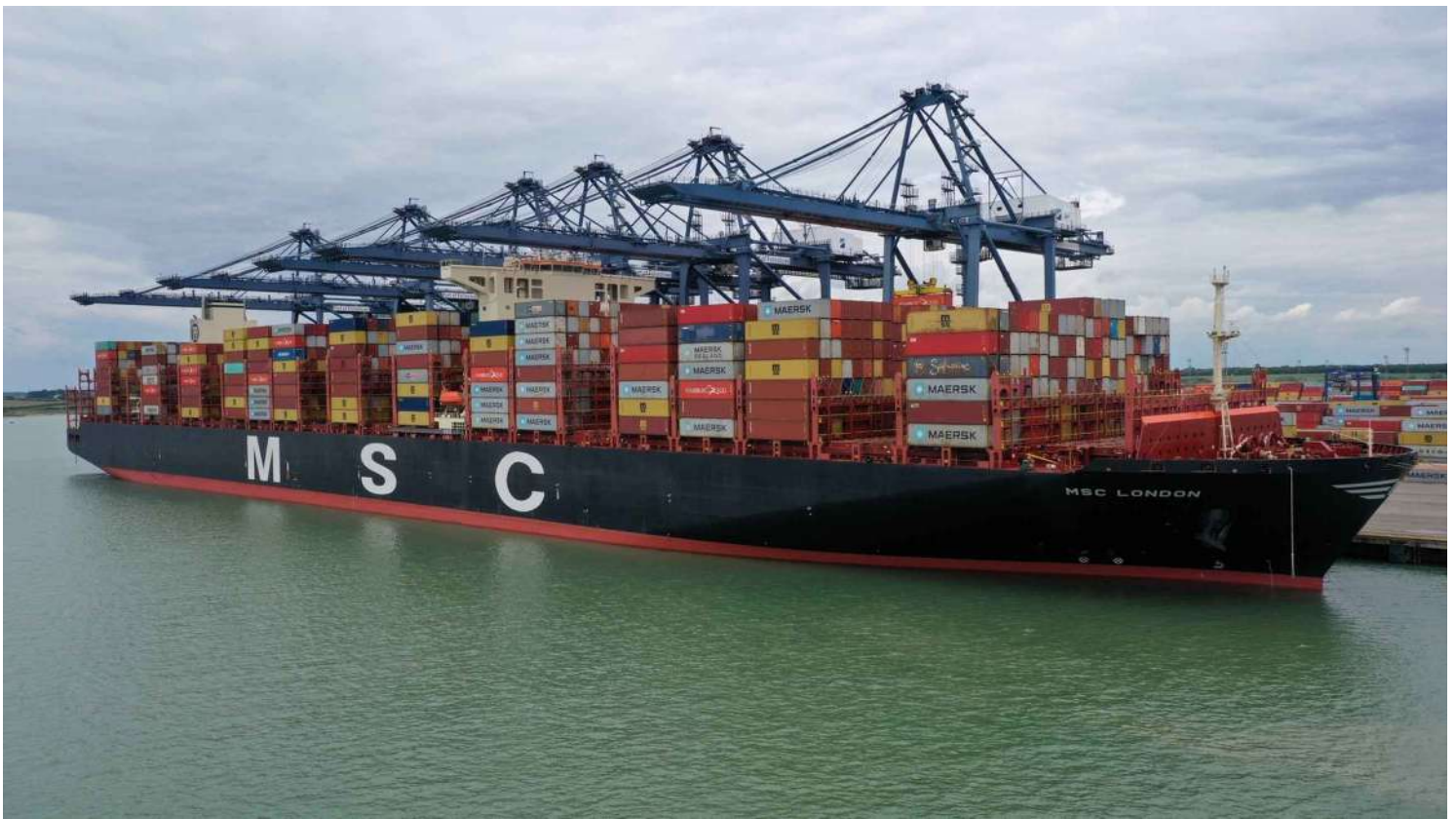
Another fairly regular caller at Felixstowe, “MSC London” alongside Trinity Seven on 12 th June. She arrived fully laden from Xiamen and Tanjung Pelepas on 10 th June and would not sail until the 16 th for Rotterdam. Built in 2014 by STX Offshore and Shipbuilding, Jinhae, South Korea, she has been retrofitted with an exhaust scrubber and a heightened bridge. (Photo contributed)
