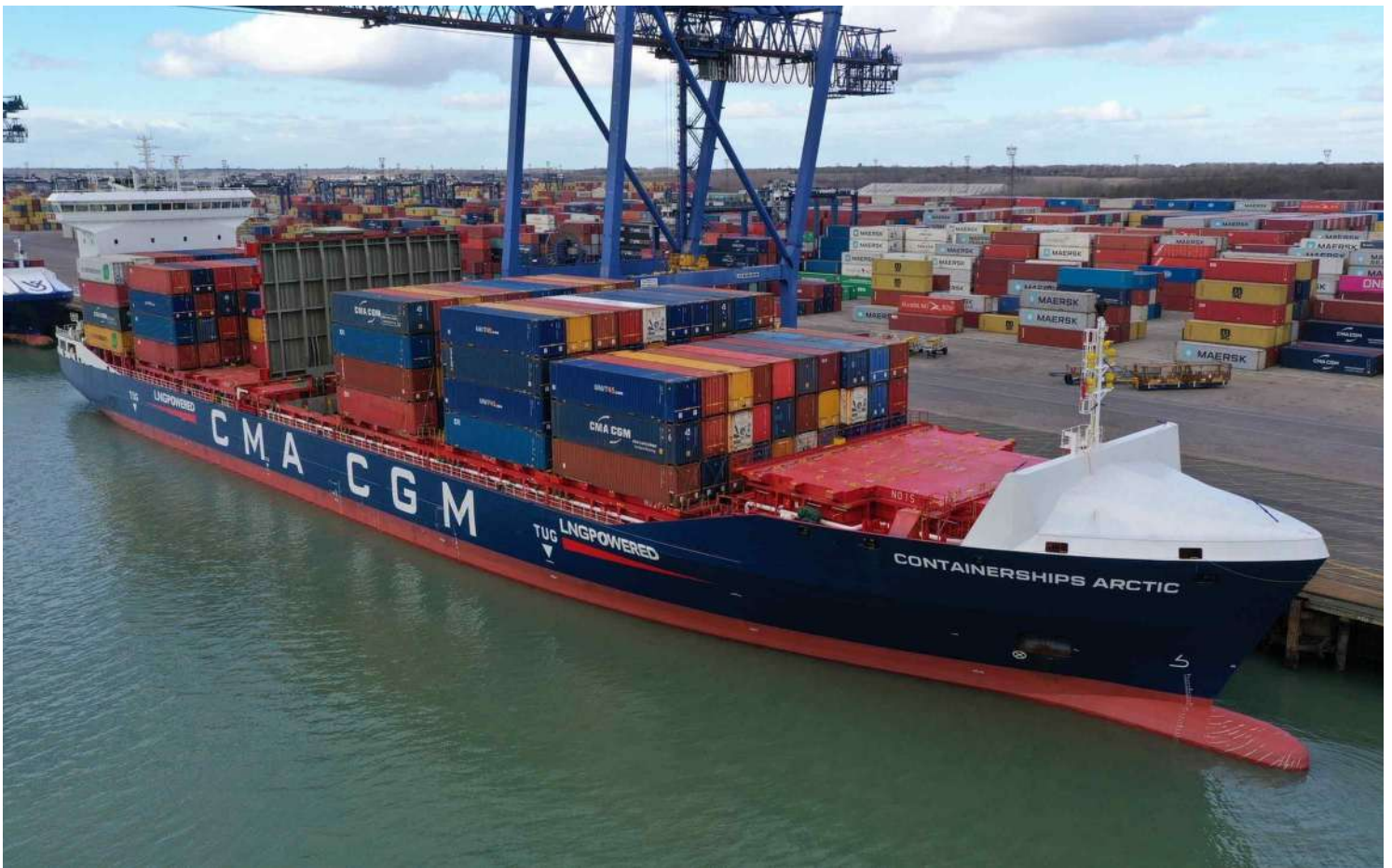
At one hundred and seventy metres and nearly 18,000 GT “ Containerships Arctic ” is somewhat large for a feeder vessel. Capable of 1,380 TEU she was built in China in 2019 by Guangzhou, Wenchong. Having arrived from Teesport in the early morning of 11 th March she would set off for Rotterdam later the same day. (Photos contributed)
