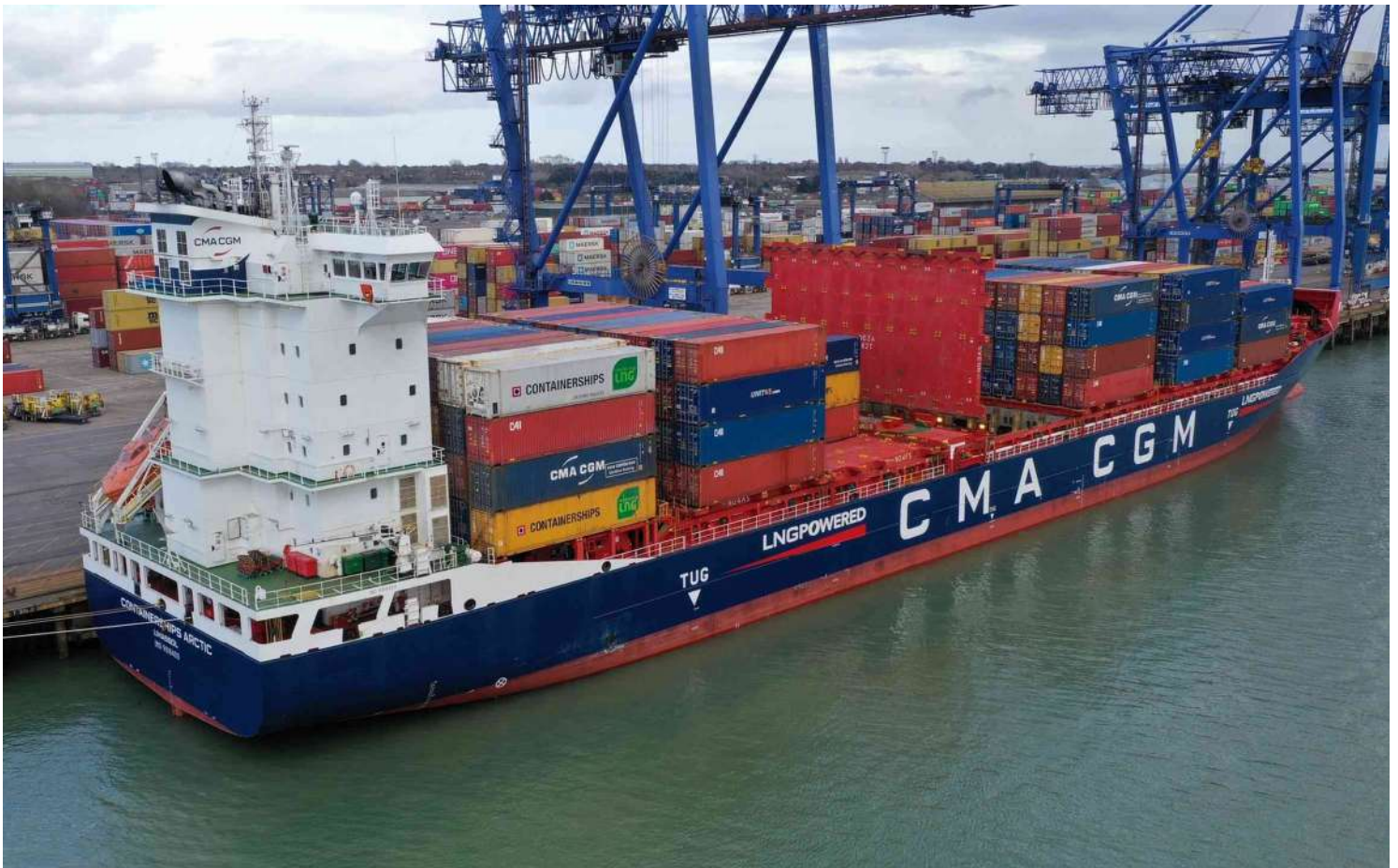
At one hundred and seventy metres and nearly 18,000 GT “ Containerships Arctic ” is somewhat large for a feeder vessel. Capable of 1,380 TEU she was built in China in 2019 by Guangzhou, Wenchong. Having arrived from Teesport in the early morning of 11 th March she would set off for Rotterdam later the same day. (Photos contributed)
